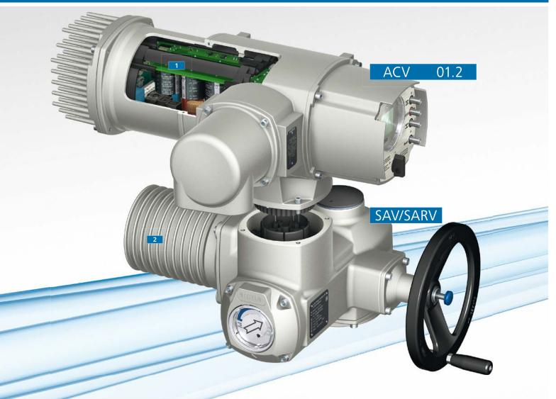
AUMA variable speed multi-turn actuators are the combination of SAV/SARV actuators and ACV 01.2 actuator controls. Variable speed is achieved by the integral frequency converter within actuator controls. ACV 01.2 are based on the intelligent AC 01.2 actuator controls. Operation and integration of ACV into the DCS is comparable to AC.
